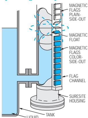
As liquid level rises, a magnet-equipped float within the unit inverts the magnetic flags in the external indicator to "color-side-out." The flags remain magnetically interlocked in a column until again inverted to "contrasting-side-out" by the float as liquid level falls. Liquid level is indicated by the junction of the "color" and "contrasting" portions of the column.
