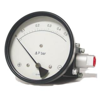
Hirlekar Precision manufactures quality differential pressure instruments designed to measure the difference in pressure between two points in a system and show it on a single dial instrument. A magnetic movement senses the differential pressure. The instrument has separate pressure and indicating chambers.
