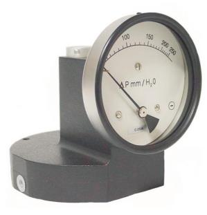
Hirlekar Precision manufactures quality differential pressure instruments designed to measure the difference in pressure between two points in a system and show it on a single dial instrument. A magnetic movement senses the differential pressure. The instruments has separate pressure and indicating chambers.
